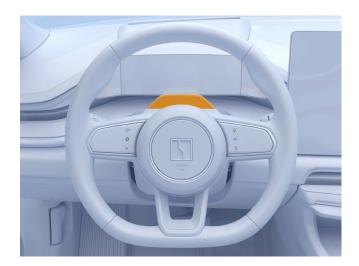
The driver detection camera is located on top of the steering wheel. The camera is equipped with low-light functionality, so it also works in low light and at night.
