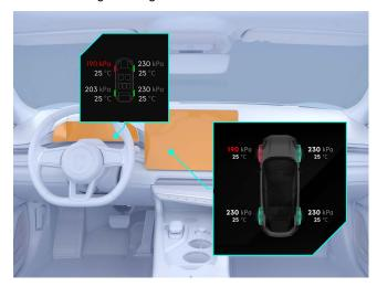
If there is an issue with the tires, the TPMS status indicator illuminates constantly, and a warning message appears on the driver and center displays. The corresponding tire symbol flashes in the driver display and turns red in the center display.
