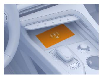
The car has a wireless charger in the front part of the tunnel console. The wireless charger can charge devices supporting the QI wireless charging standard.
