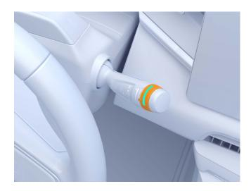
When the wiper blades are on the automatic function use the thumbwheel to adjust the sensitivity and frequency. Upwards increases the frequency of the wipers, downwards decreases the frequency.
