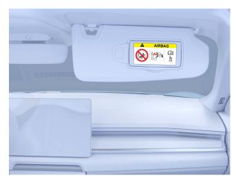
There is a warning label on each side of the sun visor of the front passenger seat to remind you to deactivate the front passenger airbag when using a rearward facing child seat on the front seat.
