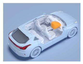
The front passenger airbag is located behind the panel above the glove compartment. Its location is indicated by the AIRBAG marking on that same panel.
