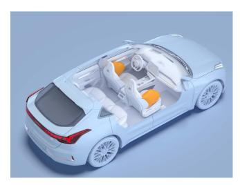
The front side airbags are located in the outer backrest frames of the front seats. Their location is indicated by the AIRBAG marking on the tags on these frames.
