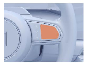
5 Press and hold the top/bottom/left/right area of the touch pad on the right side of the steering wheel to adjust the position. The corresponding arrow symbol on the heads-up display becomes green and the mirror moves in the same direction.
