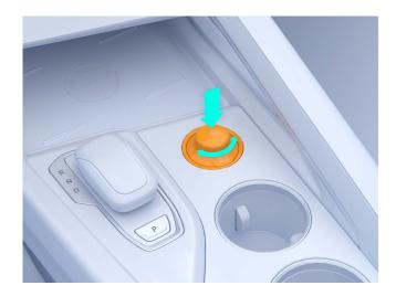
To quickly control the music, use the volume knob on the tunnel console instead of the center display. The volume knob is used in the following ways:
