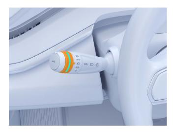
The dial near the outer end of the left stalk is used to turn on/off various lights used during driving. Rotate the dial to cycle between the indicated light functions. Rotating the dial to 0 deactivates all exterior lights except daytime running lights. See the table below for a description of each light function.
