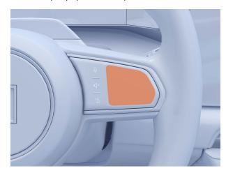
4 Press and hold the top/bottom/left/right area of the touch pad on the right side of the steering wheel to adjust the position. The corresponding arrow symbol on the heads-up display becomes green and the steering wheel moves in the same direction.
