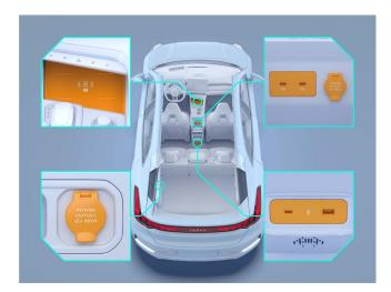
The car has several power outlets, and a wireless charger for powering and charging electrical devices:
