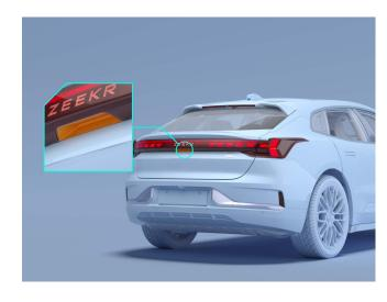
When the vehicle is unlocked, press the button on the tailgate to automatically open the tailgate. The lights in the luggage compartment and the rear position lights automatically turn on when the tailgate is opened.
