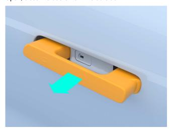
To open the door, pull the door handle that automatically pops out when the car is unlocked.
