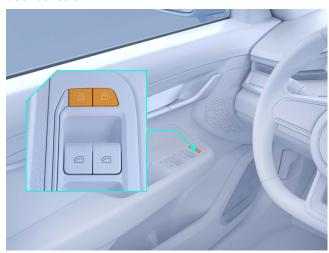
The doors and windows can be controlled with the buttons on the driver door console.
