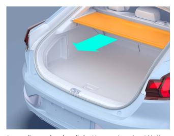
A concealing panel can be pulled out to prevent people outside the car from seeing the contents of the luggage compartment. Nothing heavier than light clothing should be put on top of the concealing panel. If the concealing panel interferes with the top tether straps for the rear ISOFIX seats, it can be removed by pulling the panel straight out.
