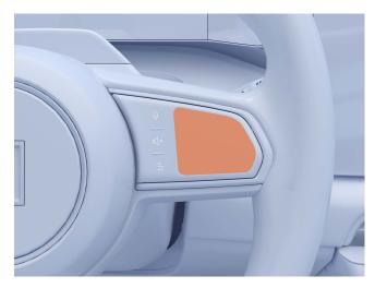
The edges of the touchpad on the right side of the steering wheel are used to adjust the heads-up display settings:
