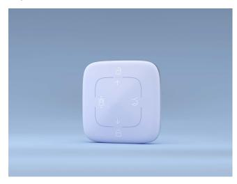
The key fob can be used to unlock and lock the car, open the tailgate, control the windows and remotely drive the car into and out of tight parking spaces.
