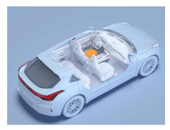
The far side airbag is located on the inner backrest frame of the driver seat. Its location is indicated by the AIRBAG marking on the tag on this frame.
