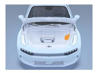
2 Remove the washer fluid cover.
