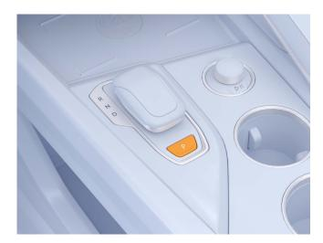
To activate the parking brake, press the P button on the gear lever when the car is powered on and stationary or navigate to —-Driving.
