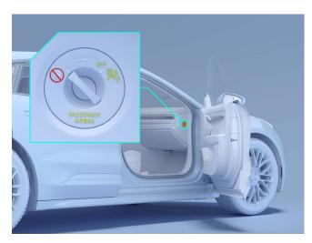
The passenger airbag switch is located on the passenger end of the instrument panel and can be accessed when the passenger door is open.
