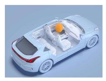
The front driver airbag is located in the center of the steering wheel. Its location is indicated by the AIRBAG marking on the steering wheel.
