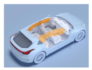
The inflatable curtains are located along both sides of the roof lining. Their locations are indicated by the AIRBAG marking on the trim panels.
